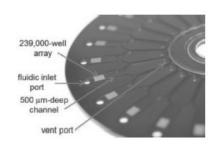
Injection of Bead/Substrate Solution into Simoa Disk This mixture of beads and enzyme substrate is then injected into our proprietary Simoa disk, which contains 24 arrays of microwells arranged radially. Each 3 × 4 millimeter array contains approximately 239,000 microwells, each of which is large enough to accommodate only a single bead.
