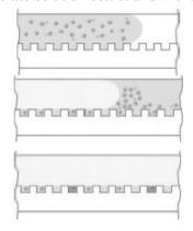
Bead/Substrate Solution Settles and Wells are Sealed The bead/substrate solution is drawn across the array and the beads settle by gravity onto the surface of the array, and a fraction of them fall into the microwells. The remainder lie on the surface, and oil is introduced into the channel to displace the substrate solution and excess beads, and to seal the wells.
