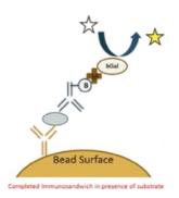
Simoa uses beads coated with capture antibodies that bind specifically to the protein being measured. After an enzymelinked detection antibody binds to the protein, the enzyme substrate is added (as depicted by the white star in the graphic on the left). The enzyme associated with the enzyme-linked detection antibody then reacts with the enzyme substrate causing the enzyme substrate to become fluorescent (as depicted by the change in color of the star in the graphic).
