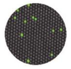
The entire array is then imaged using ultrasensitive digital imaging, and the sealed wells that contain beads associated with captured and enzyme labeled protein molecules are identified.
