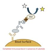
Simoa uses beads coated with capture antibodies that bind specifically to the protein being measured. After an enzymelinked detection antibody binds to the protein, the enzyme substrate is added (as depicted by the white star in the graphic on the left). The enzyme associated with the enzyme-linked detection antibody then reacts with the enzyme substrate causing the enzyme substrate to become fluorescent (as depicted by the change in color of the star in the graphic).
