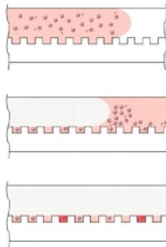
The bead/substrate solution is drawn across the array and the beads settle by gravity onto the surface of the array, and a fraction of them fall into the microwells. The remainder lie on the surface, and oil is introduced into the channel to displace the substrate solution and excess beads, and, most importantly, to seal the wells.
