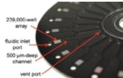
This mixture of beads and enzyme substrate is then injected into our proprietary Simoa disk, which contains 24 arrays of microwells arranged radially. Each 3 × 4 millimeter array contains approximately 239,000 microwells, each of which is large enough to accommodate only a single bead.
